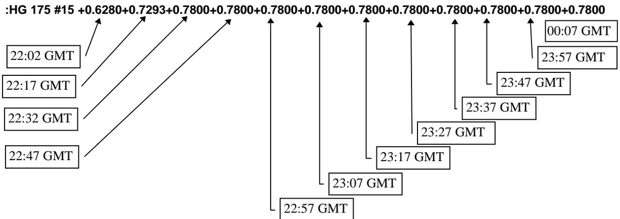
The readings on the left occurred at 15 minute intervals but the remaining readings were logged at 10 minute intervals. In this scenario a second line of readings would appear in the transmission such as:
