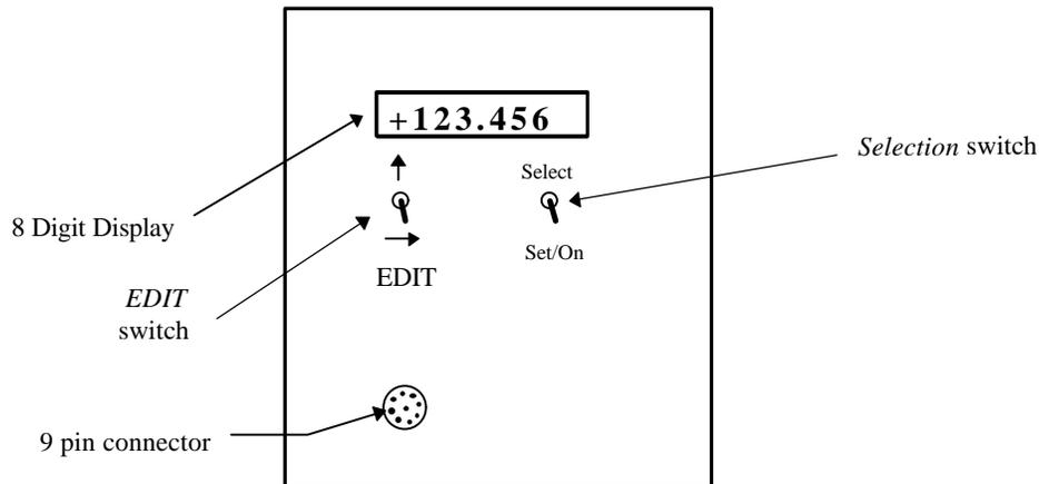
Fig.1 Front view of built-in display.
