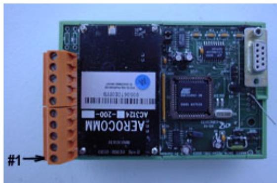
**Figure 5. Location of screw terminal #1 on the PRF.**
